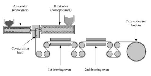
**Figure 1** Schematic of continuous tape coextrusion and solid state drawing line for the production of highly drawn polyolefin tapes possessing a high degree of molecular orientation.
