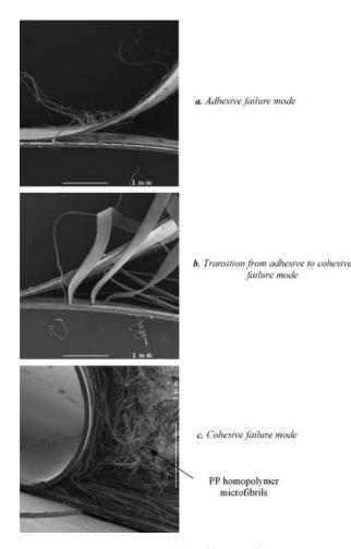
Figure 15 SEM images of different failure modes in bonded tapes showing the range of failure modes witnessed in these tests.
