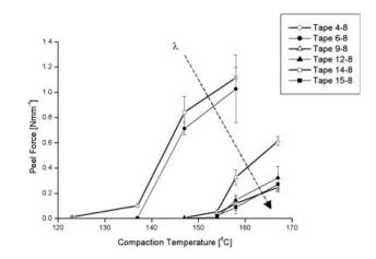
**Figure 6** Peel force versus compaction temperature for tapes with increasing draw ratio and constant percentage copolymer showing an increase in peel force with compaction temperature for all specimens but a decrease in peel force with increasing draw ratio.
