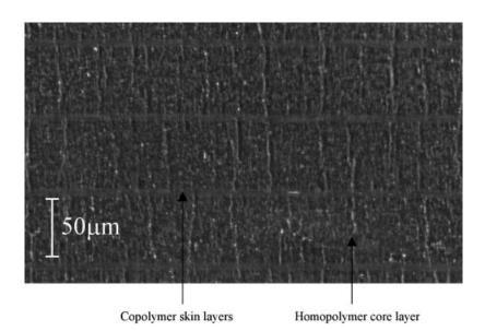
**Figure 2** Optical micrograph of a cross section of unidirectional all-PP composite showing the skin-core morphology of stacked tapes in a consolidated composite laminate (the tapes are oriented horizontally, with tape thickness oriented in the vertical direction, and tape width oriented out of the plane of the paper). The copolymer layer is clearly visible in between the highly oriented homopolymer core even within the consolidated composite.
