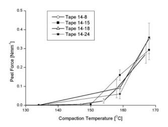
**Figure 7** Peel force versus compaction temperature for tapes with increasing layer content showing a uniform increase in peel force with compaction temperature but no significant effect of skin layer thickness on peel force.
