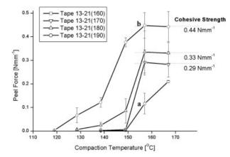
**Figure 11** Peel force versus compaction temperature for tapes with increasing drawing temperature showing an increase in peel force with compaction temperature until a maximum is reached for each drawing temperature. Samples a and b are highlighted and shown in further detail in Figure 12.
