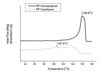
**Figure 5** DSC traces of homopolymer and copolymer used in tape production showing the broad melting behavior of the copolymer used for the skin material and the sharp melting peak of the homopolymer core material.
