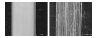
**Figure 12** Optical micrographs of peel surfaces taken from samples a (left) and b (right) as shown in Figure 11, indicating the effect of drawing temperature on tapes compacted at the same temperature. Tape a has a smooth surface, indicating adhesive failure between the bonded tapes, whereas tape b has a fibrillated surface indicating cohesive failure within the highly oriented homopolymer core.
