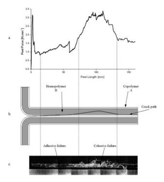
**Figure 16** Failure location of a single T-Peel specimen: (a) peel force versus peel length, (b) schematic of peel path, and (c) composite photo of peel surface with mm scale increments. These diagrams illustrate the relationship between failure mode and peel strength.
