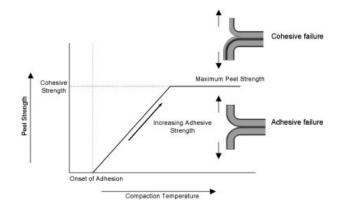
**Figure 17** T-peel failure model showing the change of failure mode from adhesive to cohesive with increasing compaction temperature.
