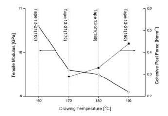
**Figure 14** Cohesive peel strength and tensile modulus of tapes drawn as a function of the drawing temperature showing that an increase in cohesive peel strength achieved by increasing the drawing temperature is accompanied by a decrease in tensile modulus.
