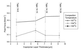
**Figure 10** Peel force versus copolymer layer thickness for tapes with increasing proportion of copolymer showing no effect of increasing copolymer layer thickness on peel force. This reveals that the increase in peel force with layer thickness shown in Figure 9 is actually controlled by changes in draw ratio rather than layer thickness itself. (Even though proportions of the tape are constant, tapes with higher draw ratio have thinner skin layers).
